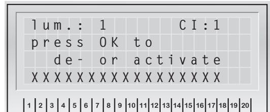
Use the navigation buttons to select the luminaire address and press "OK" to register/deregister it. You can only program registered addresses and only these will signal faults.
