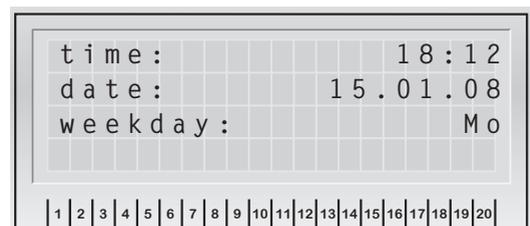
Use the navigation buttons to set the date and time of the realtime clock. Press "OK" to continue. You need to set the correct day of the week to be able to carry out automatic function tests.
