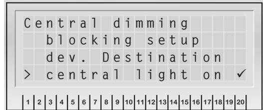
If the CLS system is connected to a CLS-MTB and the function „central light on“ is activated, all connected luminaires will switch on in the following cases:
