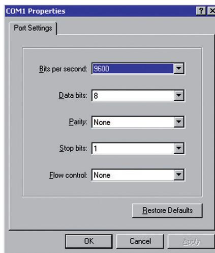
Then establish the connection settings to communicate with the InoWeb module. Enter the following values:
