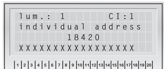
Use the navigation buttons to enter the number, then press "OK" to continue. Press "ESC" to exit the menu. After this assignment, configure the luminaires accordingly under the "Config. luminaires" menu. You can choose between 3 operating modes for each luminaire:
