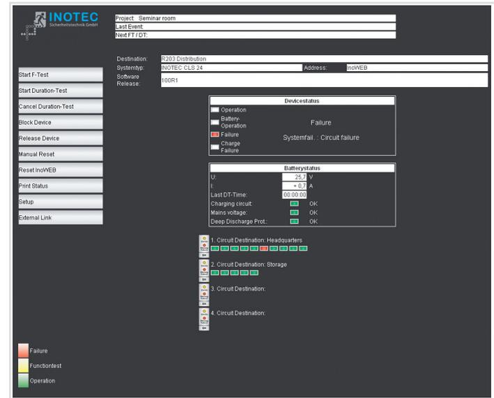
A view with all connected luminaires and their destination description is opened by clicking on a circuit.
