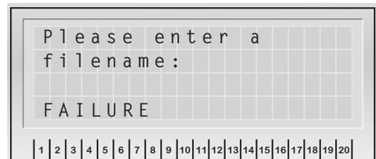
Before running the "save faults" command, connect the INOSTICK to the keyboard connection on the CLS device. After entering a file name, the entries are stored on the INOSTICK. If the file name already exists, choose a different name.
