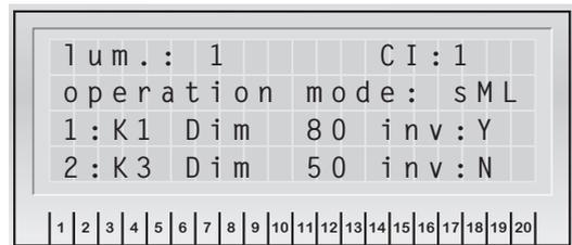
K1-K4 specify the channel for the in-system light sequence switching. Under each assignment you can specify a dimming value for the luminaires when the channel is switched on. The "inv" option inverts the input and the assignment is activated when the channel is opened.
