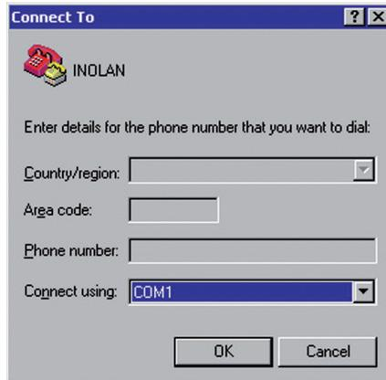
In the following dialog window, select the serial interface under "Connect using", which is used to communicate with the InoWeb module. You will need a 1-to-1 modem cable to do this.
