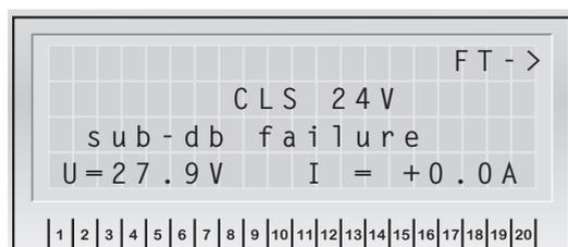
A phase monitoring system has been activated and has interrupted the current loop SL+/SL-. Check the monitored sub-distribution boards. The phase monitoring system lists the missing phases.
