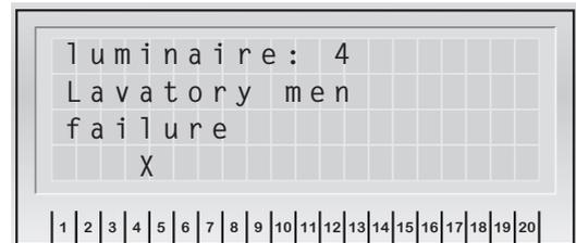
After selection of the circuit the faulty luminaires are shown with destinations. The next failure is selected with the arrow keys. "ESC" returns to the previous menu.
