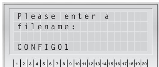
First connect the INOSTICK to the keyboard port on the CLS device. Specify a file name for the configuration file. Use the arrow buttons to select the symbol, press "OK" to jump to the next step or "ESC" to delete the symbol.
