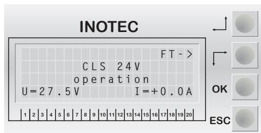
To operate the CLS system, use the 4 buttons positioned alongside the display. Use the top two buttons to navigate. Use "OK" to confirm or select a function and "ESC" to switch back to the previous menu or cancel a function.
