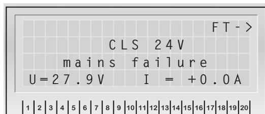
Please check the power supply. The device works in battery mode until the mains voltage returns to the input terminals or the deep discharge protection is activated.
