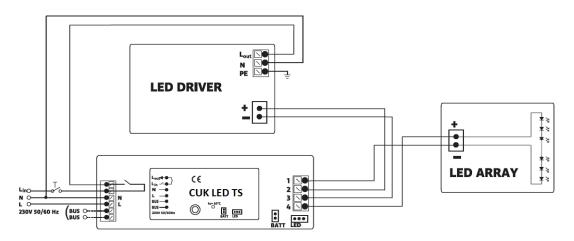
O = reinforced insulation between LED-module and mains
